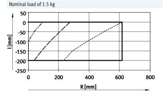
$a = 0 ... 50 \text{ m/s}^2$ - a = 80 m/s<sup>2</sup> -- a = 70 m/s<sup>2</sup> ----- a = 60 m/s<sup>2</sup>
